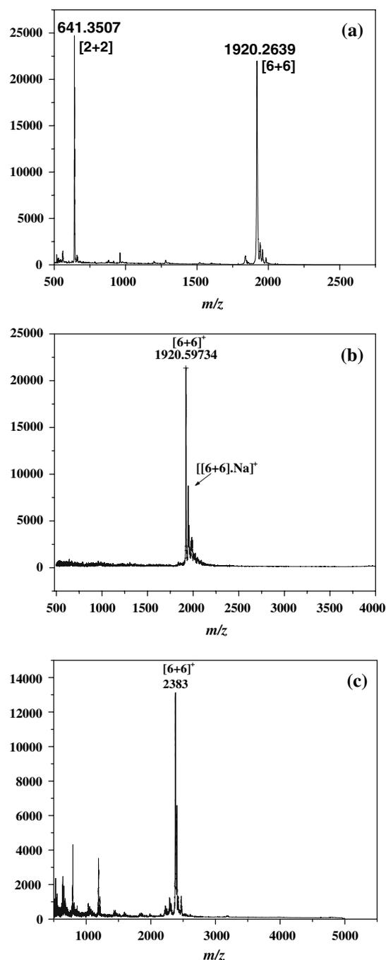
**Fig. 2** MALDI-TOF MS spectra of (a) condensation products from **3** and (1*R*,2*R*)-diammoniumcyclohexane mono-(+)-tartrate; (b) pure [6+6] macrocycle **1**, and (c) [6+6] macrocycle **2**
